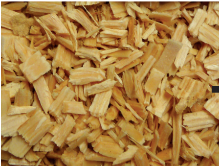
Raw material: Chips of pine, fresh from the forest, fraction 3 - 15 mm
