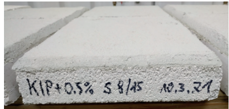
Lightweight interior lime plaster with wood chips on aerated concrete
