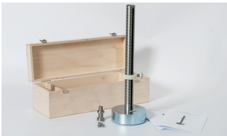
Determination of impact resistance acc. to EN 17368 for laminate floor coverings
