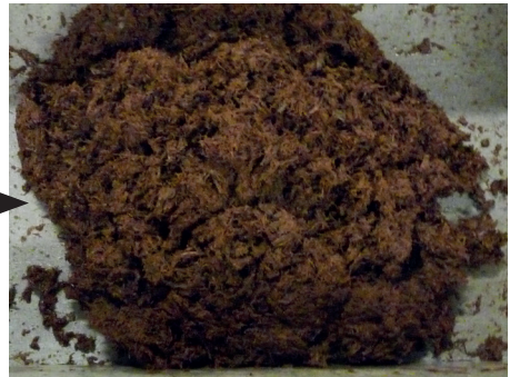
Fibre after a boiling time of 15 min at 30 bar
