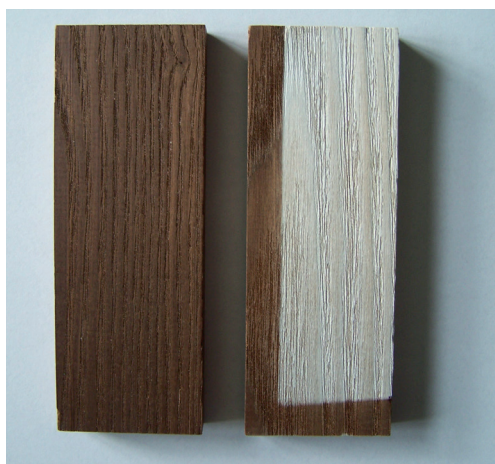
TMT ash 200 before and after 500 h of exposure in the xenon test device
