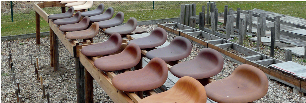
Seating elements (Gubi barstool) made of thermally modified veneers subjected to several stages of treatment, in outdoor weathering (thermal treatment by IHD and OWI, manufactured by REHOLZ)
